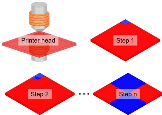
Fig. 6. The process of multipolar magnetizing by magnetic printer. The DOM is upward in red region and downward in blue region.
