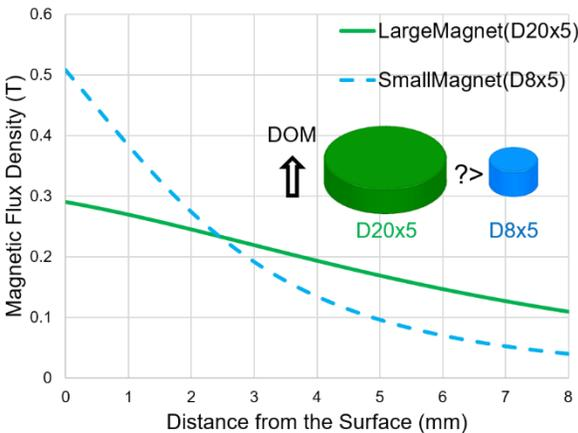
Fig. 1. Magnetic field along the axes of two cylindrical rigid PMs with dimensions of D20mmx5mm and D8mmx5mm.
