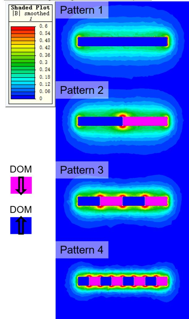
Fig. 2. Flux density distribution for Polymagnet with different patterns, the overall sizes are kept the same as 20mm\*5mm\*2mm. DOM is along with the 2mm edge. DOM is represented by the colors of blue and pink.
