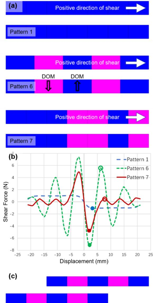
Fig. 5. The alignment behavior for a pair of Polymagnets with a certain pattern. The overall size for each sub-pattern is 20mm\*5mm\*2mm, the air gap is kept to be 1.5mm while one sub-pattern is sheared relative to the other. (a), arrangement of magnetic poles for different patterns, (b), the variation of shear force for different patterns with shear displacement, (c), one possible misalignment for Pattern 6.
