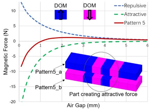
Fig. 4. The reversal of interactive magnetic force for Polymagnets with Pattern 5. The inset shows the arrangement of magnetic poles for the two sub-patterns. The overall size is 20mm\*5mm\*2mm for each sub-pattern.
