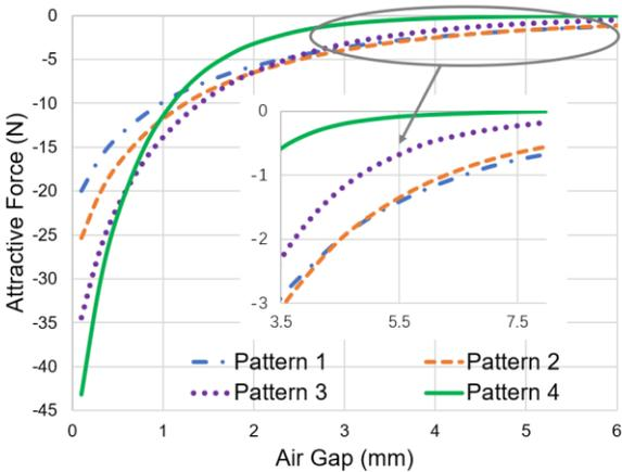
Fig. 3. The attractive force variation with air gap for a pair of Polymagnets with given pattern.
